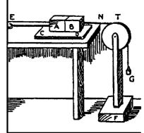
In figure 2, let F be a sufficiently strong silk thread by which marble B is attached to the floor, D a pulley, G a weight which will show the force required to pull mar-
