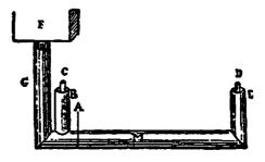
lowed the water to flow into the tube E which I had fitted up in the same way as B, and when I refilled the whole tube with water, I found that it rose to the same height in D as it had done in C. This led me to believe that the length of the tube was no hindrance, or very little.
